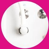
6. Attach Dome Tube onto Dome Tube Connector located on front of machine above Flow Meter.
