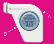
Turn on the bt-analyze by holding the power button (A) for 2-3 seconds.
